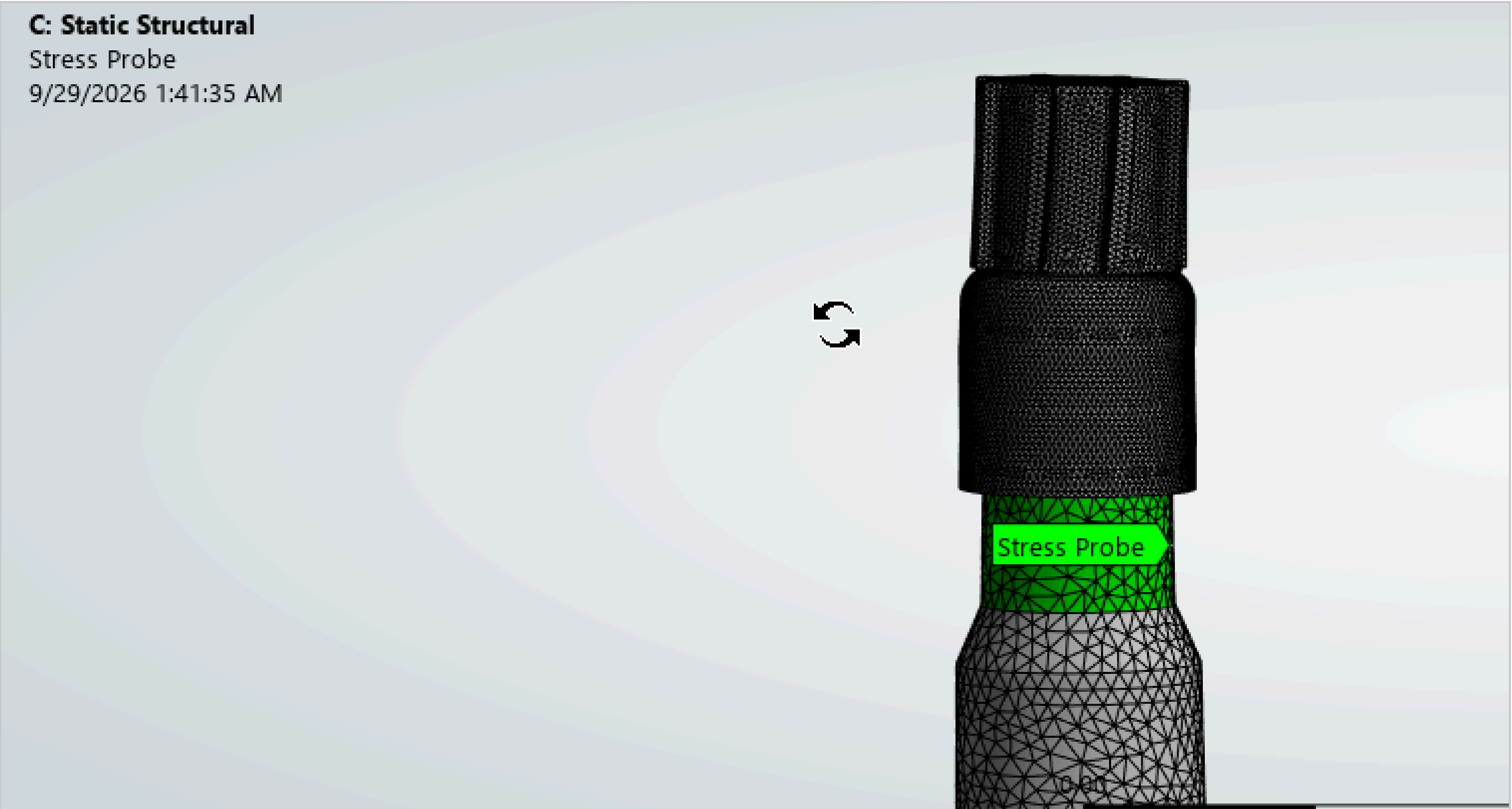
Neck probe: 206.1 MPa, 12% over nominal ( K_t \approx 1.12 ). FoS 2.67; 1.33 at \times 2 shock
